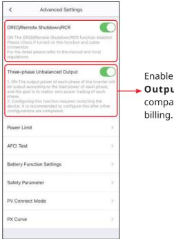
Enable **Three-phase Unbalanced Output** when the utility grid company adopts phase separate
