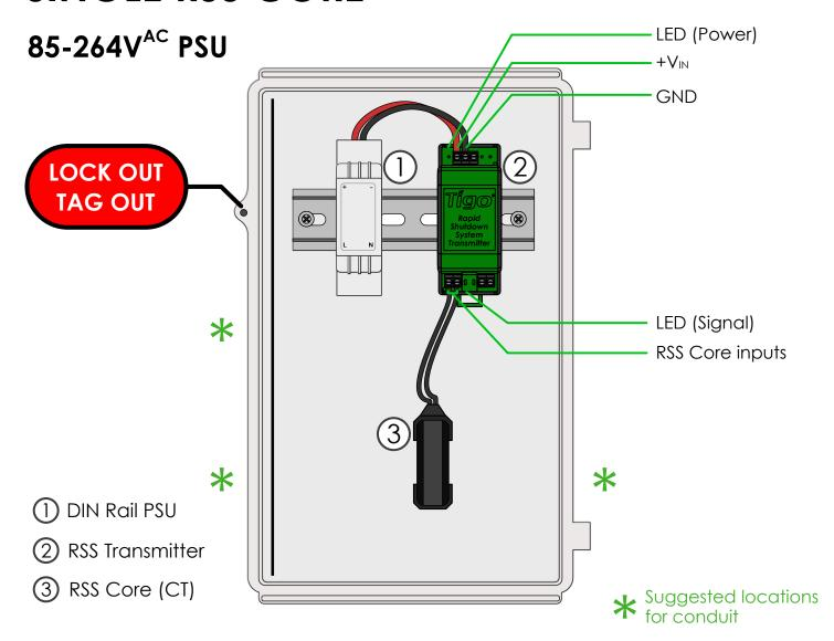
Transmitter power supply must be on same AC branch circuit as inverter to meet rapid shutdown requirements.
