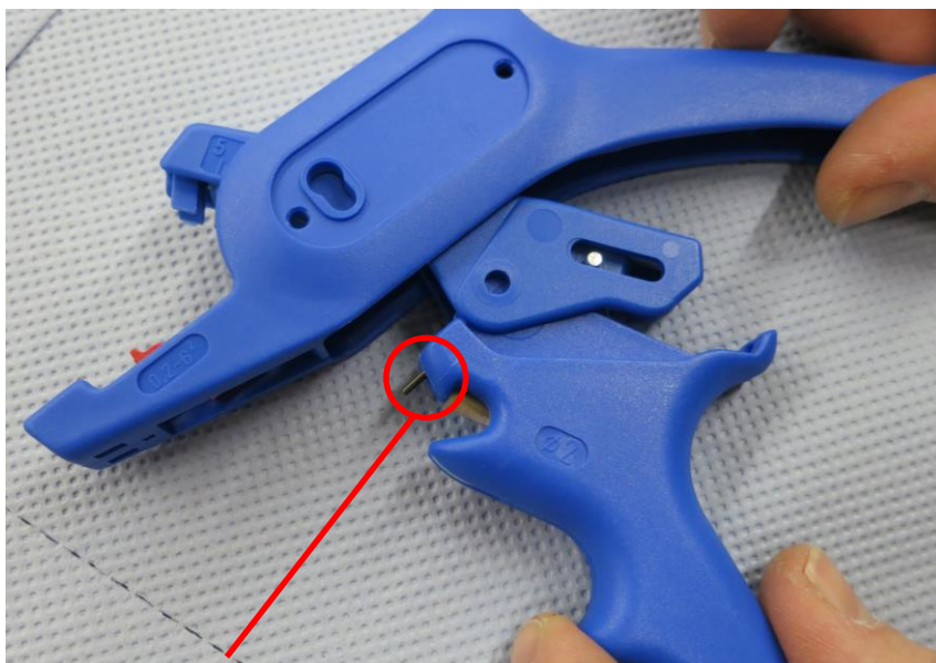
Step 8: Reinstall bottom handle component. Detailed image of steel spring
