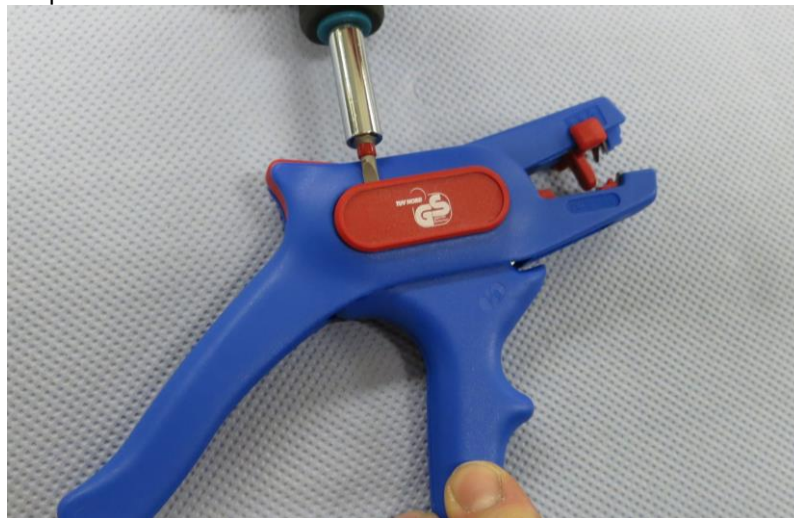
Step 2: Remove the back cover
