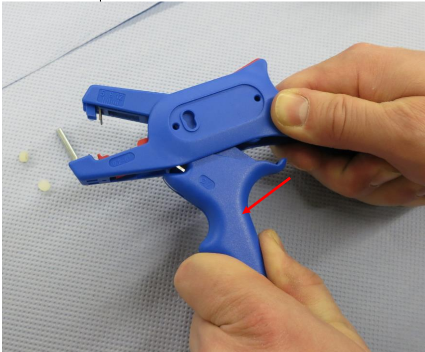
Step 5: Turn the bottom part of the handle forward
