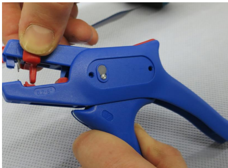
Step 3: Press the length stop together and remove by pushing downwards
