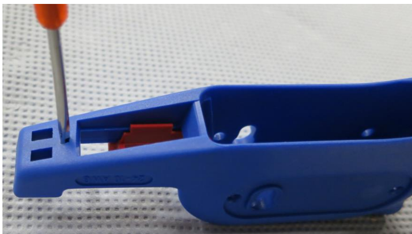
Step 7: Remove bottom blade downwards and insert new blade (possibly with weighting), it will snap into place
