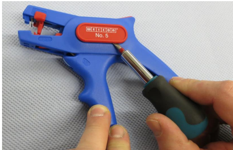
Step 1: Remove the front cover
